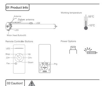
1. This product is for indoor use only, do not use outdoor or in humid environments. 2. This motor has a built-in rechargeable Li-ion battery pack with integrated charge management. Max input voltage: 5V/2A.
