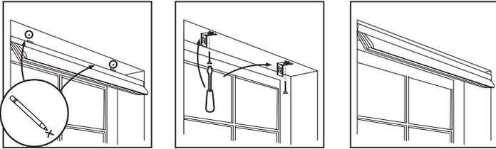
**Step 3. Securing the Headrail**
