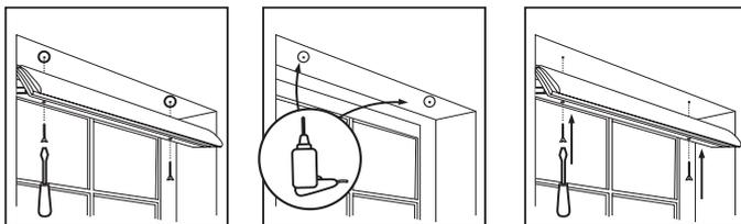
Mounting holes are pre-drilled into the headrail, so brackets are not required. Align the front of the shade with the front edge of the window opening (or position as desired), making sure the shade is centered in the window opening. **Hold the shade cloth up and over the headrail**, and then pre-drill the mounting holes using a 5/64" drill bit – screw the shade in place **using the 1-1/4" screws**. **A second set of hands makes this job much easier, so get a helper if you can.**
