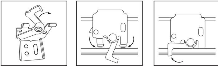
To attach the brackets the locking arm should be facing out. Then position the bracket so that it engages the inner front and inner back of the bracket. Then push the locking arm inward to lock it in place.
