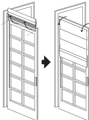
Mounting holes are pre-drilled in the headrail, so brackets are not required. Position the shade as desired over the window opening; making sure that it is level - use a Spirit Level if necessary to assure proper alignment. Hold the shade cloth up and over the head rail, and then pre-drill the mounting holes using a 5/64" drill bit - screw the shade in place using the 1-1/4" screws. A second set of hands makes this job much easier, so get a helper if possible.
