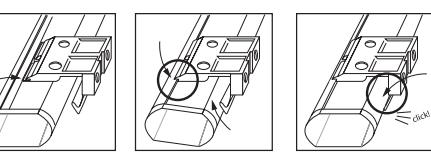
For style 'B' [see illustration]: Lift the Head Rail into position such that the front edge of the bracket is under the inner front edge of the head rail, and then push the head rail upward until the flexible tab at the bottom of each bracket snaps onto the back of the head rail. Check carefully to assure that each bracket is properly secured.
