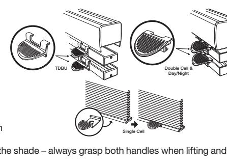
Wider shades have (2) Handles – to precisely determine the correct position for each handle, divide the total width of the shade by 4, and then attach one handle that distance from each outside edge of the shade – always grasp both handles when lifting and lowering the shade.
