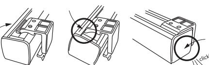
For style 'C' [see illustration]: To attach the brackets the locking arm should be facing out. Then position the bracket so that it engages the inner front and outer back of the head rail, and then push the locking arm inward to lock it in place.
