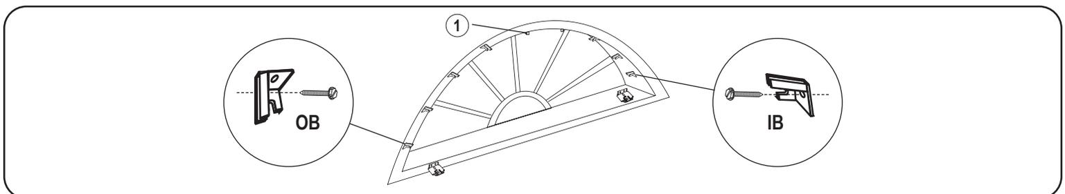
Position the clips so that the back of the clips are the same depth as the back of the installation brackets. First, place a clip at the top center of the window opening and then, space remaining clips evenly apart. Screw the arch support clips to the mounting surface through the hole in the top of the clip (IB) or through the slot in the back (OB).
