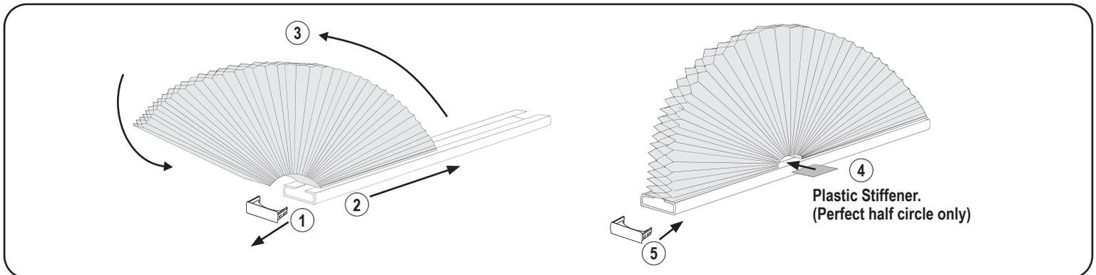
**NOTE:** Not perfect half circles have a straight edge on one end of the fabric and the other has a trimmed (jagged) edge. Orient the fabric so that the trimmed (jagged) edge, when fanned out, will become the outside edge of the arch. The straight side of the fabric stack will form the inner circle of the arch.
