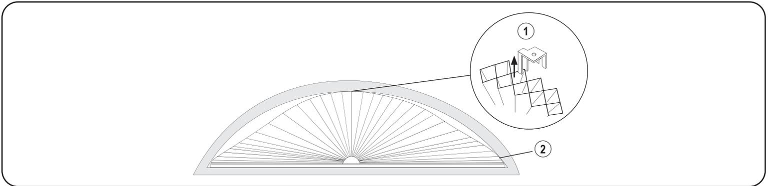
First, find the center of the fabric. Gently press on the fabric until you are able to get the back cell into the top center support clip. Then, go to the first clip up from the bottom of the arch and gently lift and fan out the fabric until the first section fits the window opening. Gently press on the fabric until you are able to get the back cell into the support clip. Repeat for remaining clips. Check the fit of the arch shade. Reposition the fabric in the clips, if necessary.
