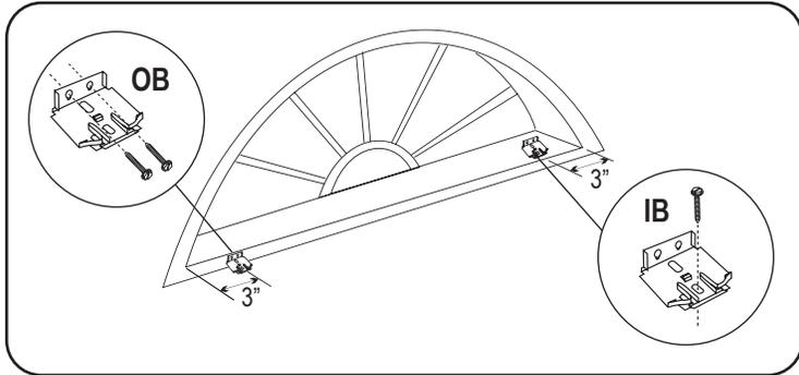
Mount end brackets 3" from each side and space any remaining brackets evenly. Make sure that all brackets are aligned and level. For the best fit on a non-perfect half circle in a deeply recessed window opening, position the brackets so that the arch is installed close to the original depth that the template was made.
