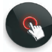
(5) Press and hold the central button on the hub until the circular light turns RED and Flashes
